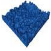
These reverse osmosis membranes are layers of material with an active aromatic polyamide layer that allows water molecules through, but screens out 99 to 99.9 percent of the salt. Gomez and his team looked at the internal structure of the polyamide film using high-angle annular dark field scanning transmission electron microscopy (HAADF-STEM) tomography. "We found that the density of the polyamide layer is not homogeneous," said Gomez.
