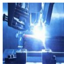
(A bed of additive-manufactured titanium components for the Boeing 787 Dreamliner. Photo via Norsk Titanium) A bed of the first RPD produced titanium components for the Boeing 787 Dreamliner from 2017. "Integrating additive manufacturing capability into our production system to build end-use titanium parts expands Spirit's fabrication capabilities and puts us at the forefront of advanced manufacturing," commented Kevin Matthies, Spirit AeroSystems senior vice president of Global Fabrication.
