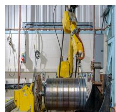
The titanium pressure vessel was produced by Wire Arc Additive Manufacturing at Cranfield University. Eng Massimo Chiampi, Study Manager for Additive Manufacturing projects at Thales Alenia Space, stated, "We were looking for an innovative manufacturing solution for the tanks, which typically suffer from long lead time with the conventional production route based on subtractive machining."
