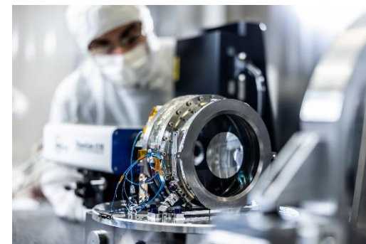
Integration of SEEING 130 Wide for micro/nano satellites
