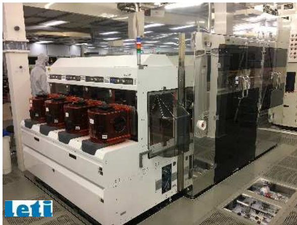
Alignment using an EVG Gemini FB XT and a SmartView®NT bonder
